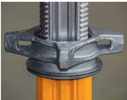
The design of the impact cam on the adjusting nut provides the direction, which is hit using a hammer in order to release the load.
