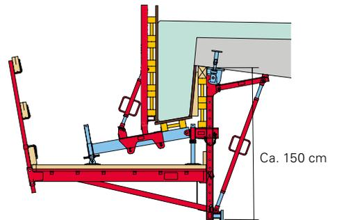
The VGK Cantilevered Parapet Bracket has another area of application. It can also be used as a working platform in building construction and civil engineering. The same components are used for these applications.
