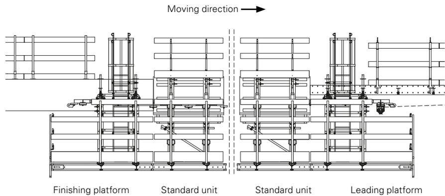
The rollers to be freed up are dismantled from the finishing platform and re-mounted in the moving direction at the front from the leading platform.
