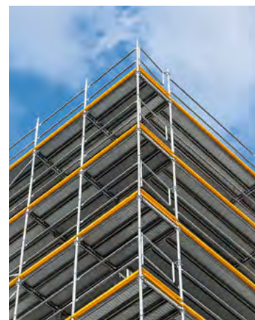
To form outside corners, you only need a frame column – all you then have to do is fit your decks on the horizontal ledger of the adjoining scaffolding bay.
