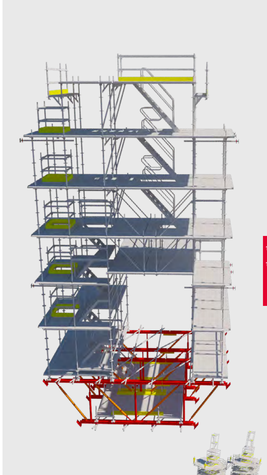
3D planning facilitated assembly in the narrow and dusty chimneys and helped the scaffolders to find their way around.
