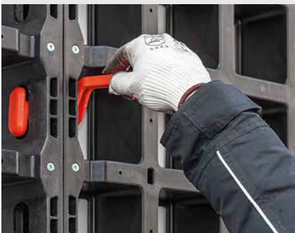
The DUO coupler is simply inserted through the elongated frame openings and then turned through 90° to secure it in place.
