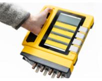
The recorded data is sent to the ISC Hub via the ISC Node. The measurement results are shown immediately on the ISC Hub display.
